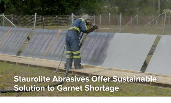
hough many may think of garnet as just a beautiful gemstone, the mineral is also used extensively for industrial purposes. When bridges, water tanks, or buildings need to be cleaned and prepped for weather-proof painting, abrasive (sand) blasting is most commonly used. To cut steel, rubber, glass and other materials, abrasive waterjet cutting is employed. Both techniques use compressed air or water to propel abrasive particles of sand to clean or cut through tough surfaces.
