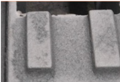
Gray Iron Silica Sand Casting showing burn-in
